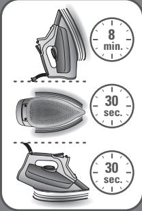
**EN** When plugged, the iron will automatically switch off after: 30 seconds when left on the soleplate or side; 8 minutes when left on its heel.
