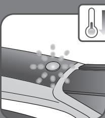
**EN** When Auto Off function is on the Auto Off indicator light blinks and the iron starts to cool down.
