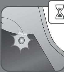
**EN** The pilot light is switched on when the iron is heating up.
