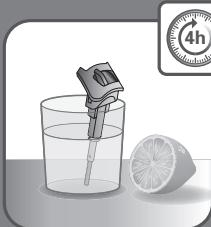
**EN** Soak the anti calc valve in a cup of plain lemon juice or a cup of white vinegar for 4 hours. **WARNING:** never touch the end of the valve.
