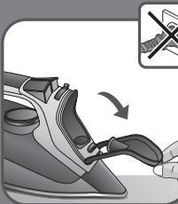
**EN** Open the filling inlet door (the iron is unplugged).
