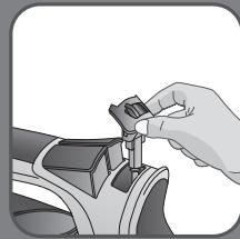
**EN** Release valve pin to the self clean position and keep it in the raised position.
