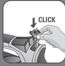
**EN** Replace the anti calc valve into position.
