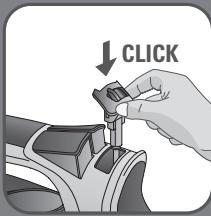
**EN** Replace the anti calc valve. **WARNING:** the iron will not function without the anti calc valve.
