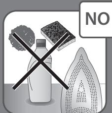
**EN** Do not use detergent to clean the soleplate. We recommend the Rowenta soleplate cleaning kit. Do not use sharp or abrasive cleaning accessories to clean the soleplate.
