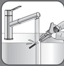
**EN** Rinse the anti calc valve under running water.
