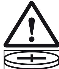
The battery included in this product is not user replaceable. Consumer shall never attempt to replace the battery. Compatible battery type is: CR2450. Nominal battery voltage is: +3.0V.
